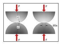
• For analysis, this can be reduced to two spheres and can be mathematically modeled using Young's Modulus and Poison's theory to functions of material properties of resistivity.
