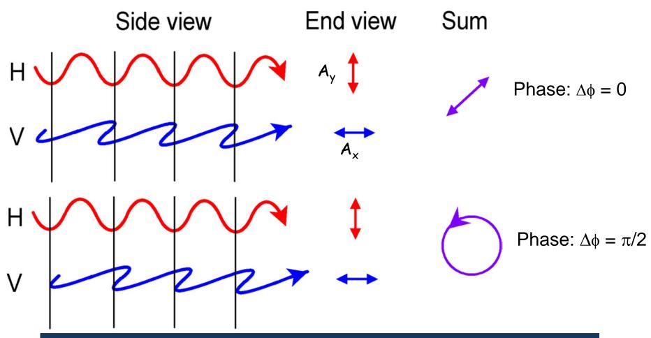
Relative amplitudes  $A_x$  and  $A_y$  determine axis orientation ( $\psi$ ).
