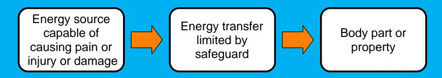
Energy is not always the hazard, it may be current or charge The unsafeguarded "Energy" is classified into three levels
