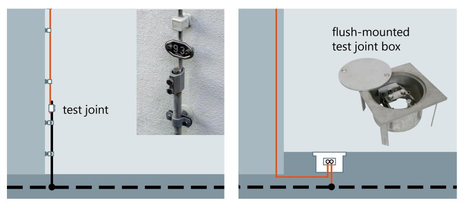
Ref.: IEC 62305-3:2010, 5.3.6 © 2016 DEHN + SÖHNE / protected by ISO 16016 **Protection measures against** touch and step voltage
