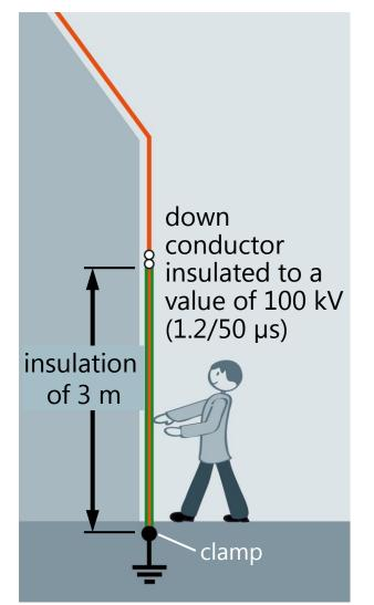
If none of these conditions is fulfilled, protection measures shall be adopted against injury to living beings due to touch voltages as follows:
