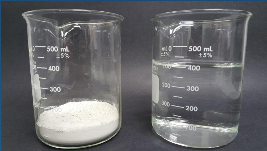
Manufacturers Mixing Instructions: 1 part Bentonite : 4 parts Water
