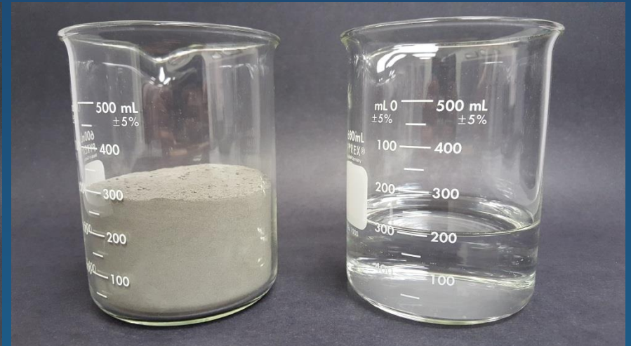
Manufacturers Mixing Instructions: 3 parts Conductive Cement : 2 parts Water
