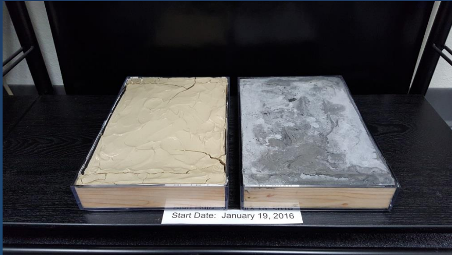
Day 3 – Shrinking & Cracking
