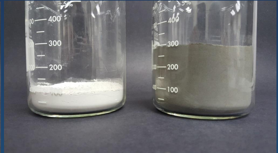
100 mL Bentonite & 300 mL Conductive Cement
