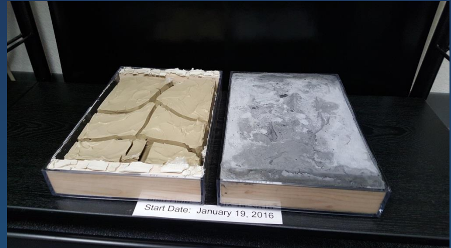
Day 13 – Extensive Cracking
