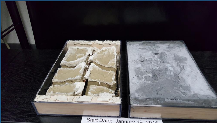
Day 15 – Electrode Completely Exposed & Crystals Start to Form
