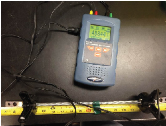
Figure 1: Mirco-ohm meter – Resistance Measurements
