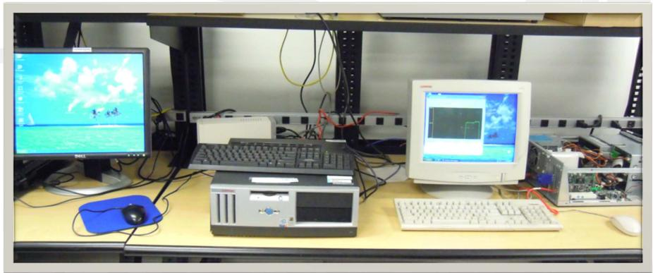
Transferring data files from one computer to another computer. Monitoring the file transfer with windows task manager. Computer # 2 opened up for NIC card insert / remove capability.
