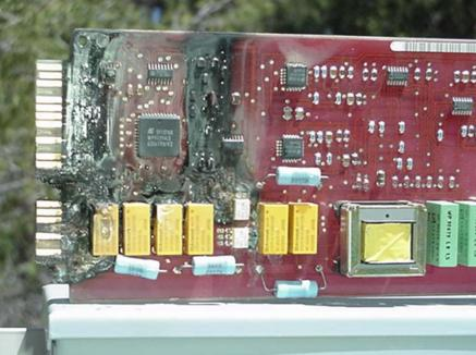
Loop Electronics can also be damaged by lightning surge currents entering through the ground system of the REC. Primary protection may "back fire" allowing those currents to pass into system components.
