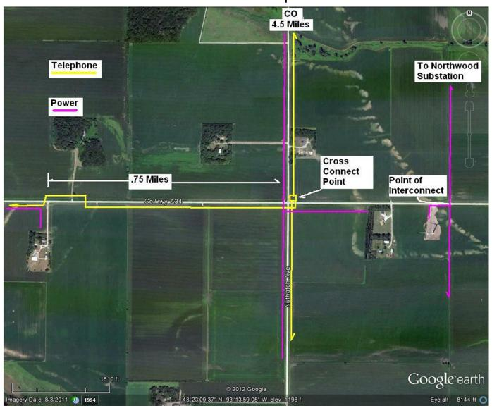
Very basic power distribution system . By design, the substation is the "power source" .
