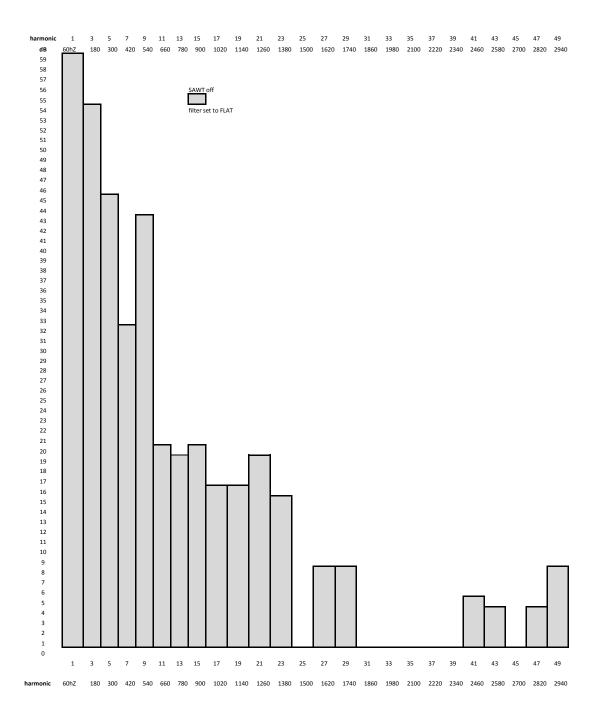
Harmonic graph with cable pair data taken with a spectrum analyzer and FLAT filtered from customers serving terminal. Stand alone wind turbine generator is ON line.
