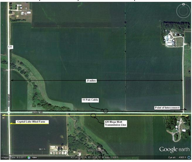
Looking east on 340<sup>th</sup> Street, transmission line on right, buried phone cable on left No "local" power distribution system to provide MGN bonding.
