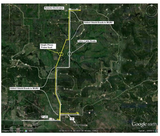
What <u>NOT</u> to bond to! Collector system is a three phase delta power system with an intersystem bonding/ static wire which is bonded to a ground electrode at every pole.
