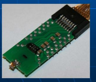
Sealing the Smith components to try and combat isolation breakdown.
