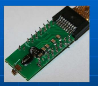
Common to see chip resistor arrays that fail during longitudinal surges.
