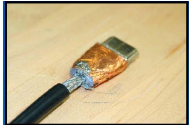
Cable braid soldered to copper foil, foil soldered to connector shell
