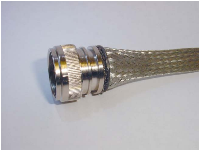
Cable braid soldered to copper foil, foil soldered to connector shell
