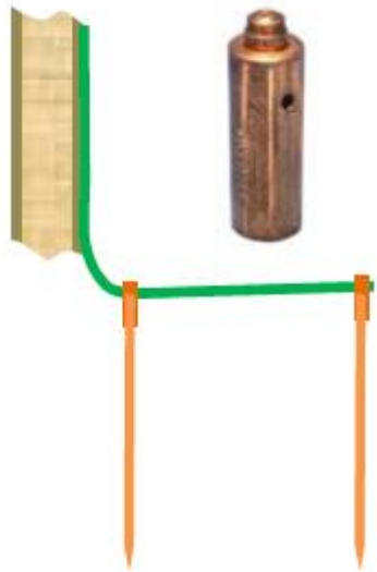
Two Ground Rods in Line
