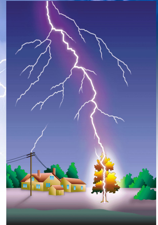
Upward leader propagates toward down leader to complete ionised path between cloud & ground
