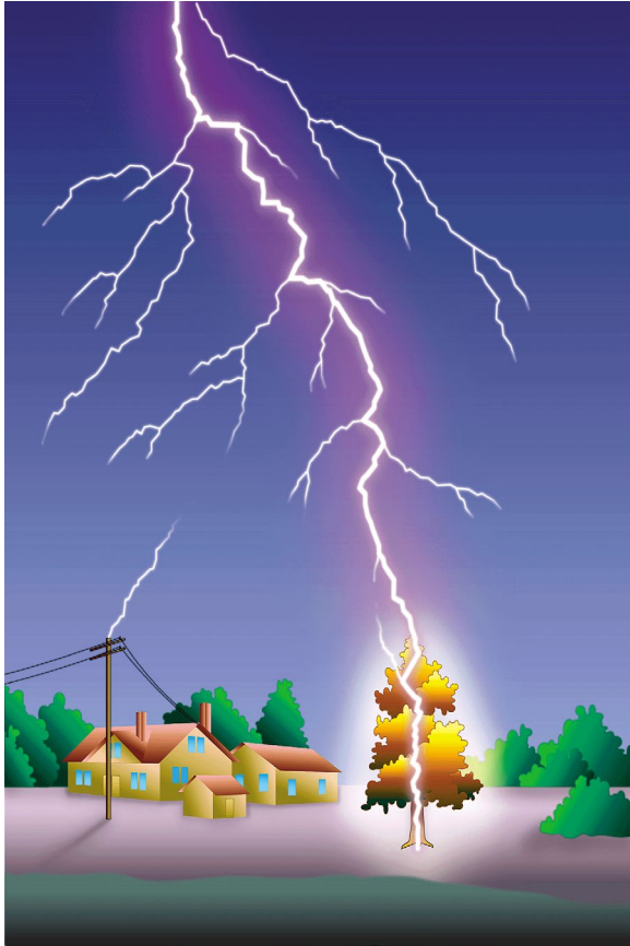
Upward leader propagates toward down leader to complete ionised path between cloud & ground
