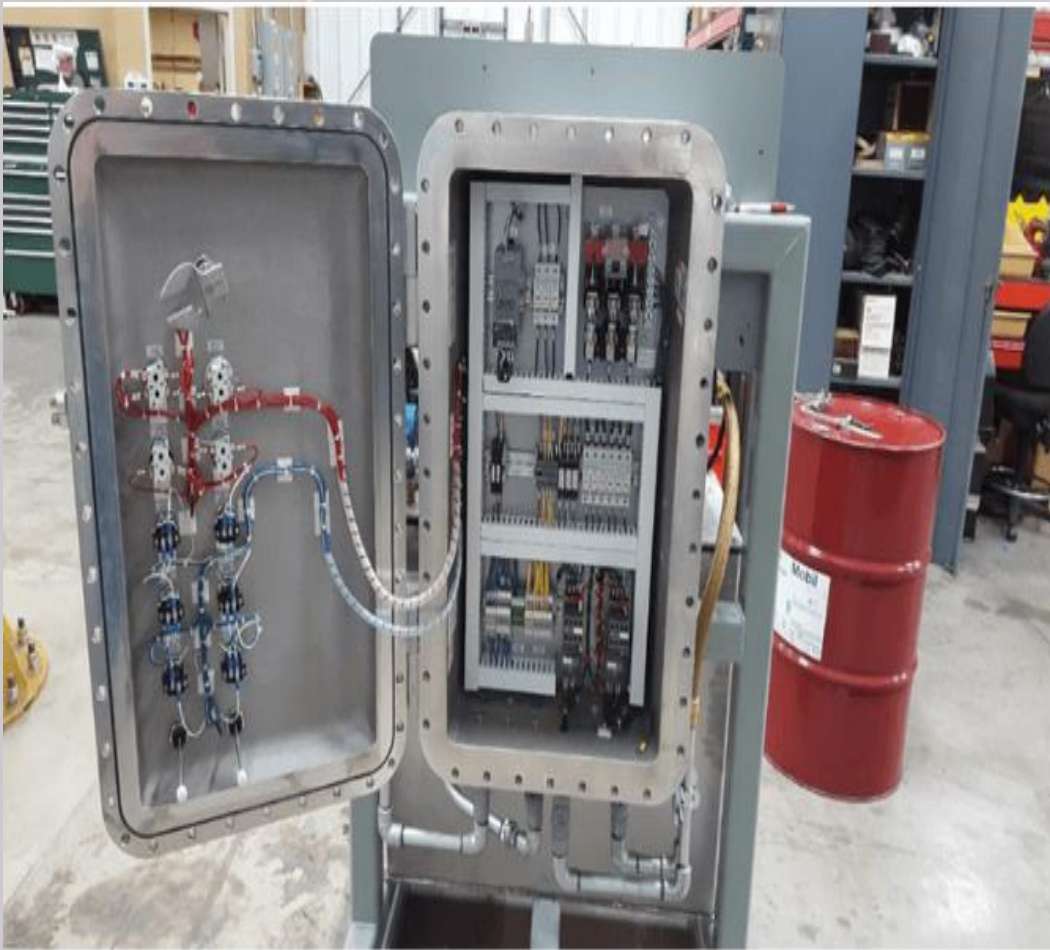
90~265 vac input & 12/24/48 vdc output UPS with LiFePO 4 battery designed for use inside NEMA 7 (explosion-proof) rated enclosure
