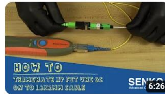
How to Terminate XP Fit Uni SC on to 1.6x2mm Cable
